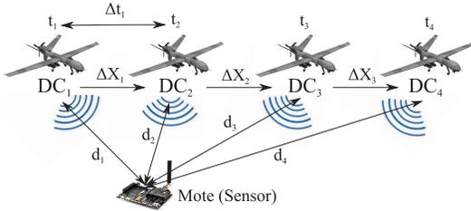
Fig. 2. Sample signal coverage model for four detected coordinates (DC) assisting mote localization.
