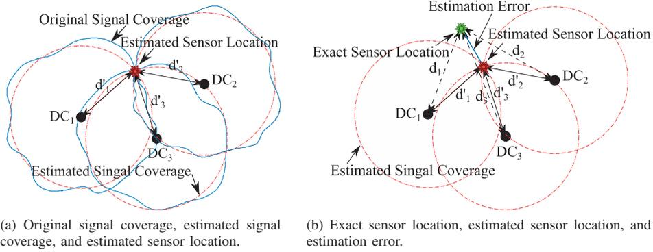
Fig. 4. Sample signal coverage model for three detected coordinates (DC) in a 2-D environment.
