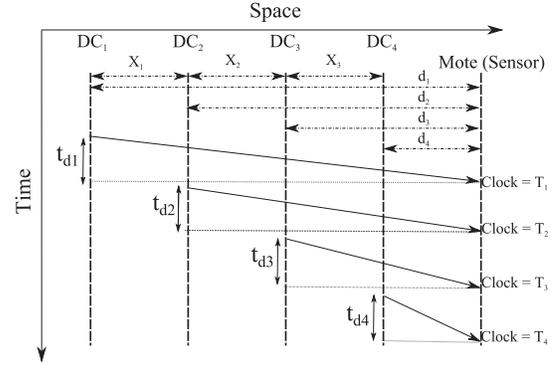
Fig. 3. Timing-diagram of packets arrival from four detection coordinates (DCs) to the mote.
